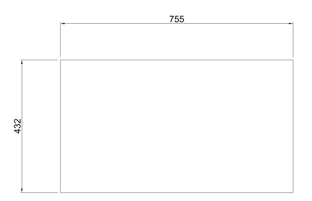
\* Cut-out template is for Drop-In (Topmount) installation ONLY. For undermount installation please email info@zomodo.ca to request a CAD (.dwg file)
