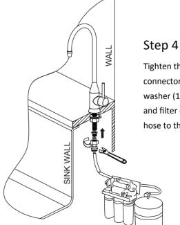
Tighten the converter (12) and filter connector (14) with a wrench, ensure washer (13) is between the converter (12) and filter connector (14). Then connect filter hose to the filter connector(14).
